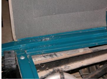
A hole was then drilled through on each side. Same for the cross member. Measure to the center and drill a 1/2" hole there as well.
