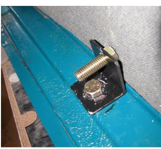
The brackets on the side are bolted through the body sill using the 4" reinforcing straps underneath. You have to get creative in getting your fingers in under the body (from the outside above the running board), holding the strap in place, getting a bolt down through and then getting a lock washer and nut started onto the bolt. Sandra as a third hand worked wonderfully!
