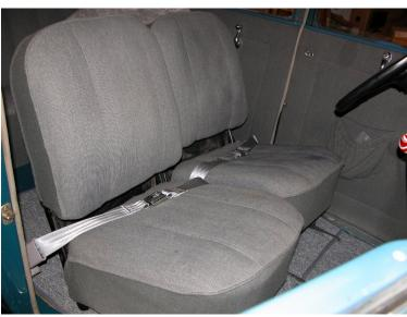
Once you have the seats back in, have someone sit in each set and adjust the angle of the retractors so that the belt pulls straight out of the unit, then tighten their attachment bolts.
