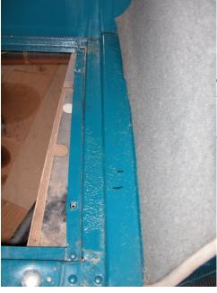
The outer ends (the end with the retractors) are mounted to the body sill. I measured a point 14" forward of the face of the rear seat and made a mark. (Well, actually, I made two, but the first one was too far forward. : -))
